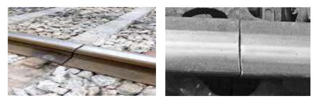
As per figure no 1 it has been observed that when online camera detected the image of railway track there was no crack but in continuous successive scanning minor cracks has been detected and related feedback has been given to the central room.
