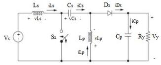
Fig.1 Proposed SEPIC converter schematic diagram.
