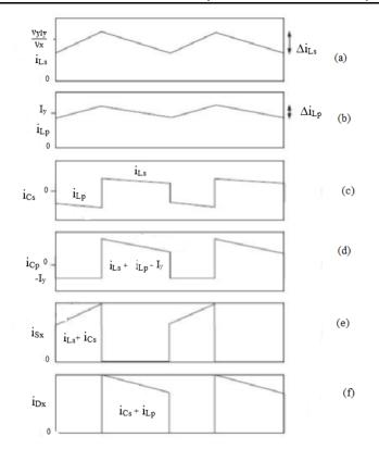
Fig.4 a. Current through Inductor Ls (iLs), b. Current through Inductor Lp (iLp), c. Current through Capacitor Cs (iCs), d. Current through Capacitor Cp (iCp), e. Current through switch Sx (iSx), f. Current through diode Dx (iDx).
