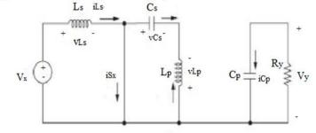
Fig.2 SEPIC Circuit with the switch closed
