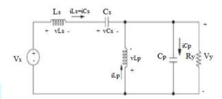
Fig.3 SEPIC Circuit with the switch open
