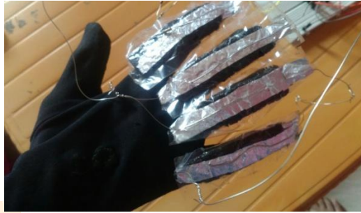
Figure 4.2.2: Flex sensor attached to glove
