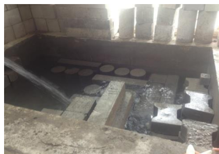
Figure 2. Curing of Specimen
