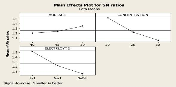
From the above graphs, we can conclude that for NaOH at 40V and 30% concentrationof the electrolyte gives minimum DOC
