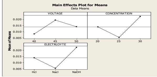
From the above graphs, we can conclude that for NaOH at 45V and 30% concentrationof the electrolyte gives the maximum MRR
