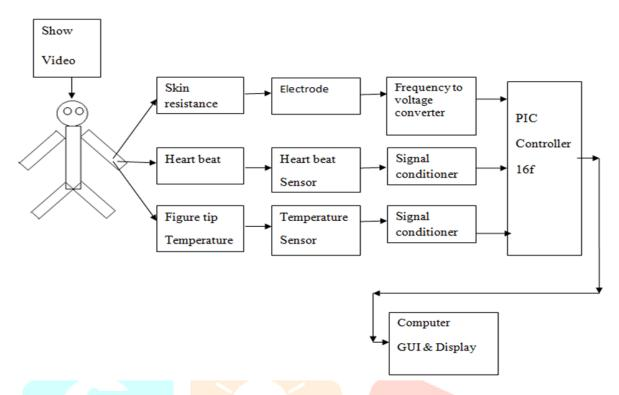
To measure body resistance, constant DC current of few microamperes is passed through the body. The voltage drop across the body is measured. The body resistance is obtained from applied constant. Current source. The constant current signal is injected in human body by source electrodes, then the voltage drop across the body is taken by sensing electrode and then voltage across human body is given to ADC of microcontroller. This voltage value is mapped to resistance using this mapping system.
