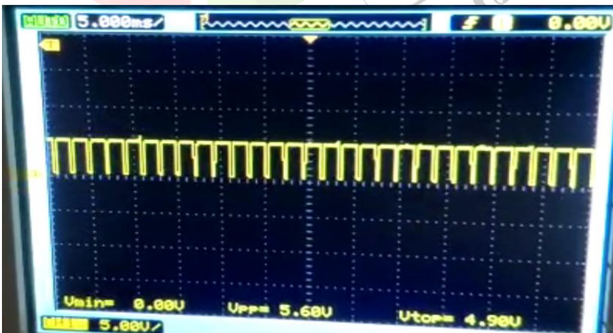
Image 9- output voltage waveform of boost converter for soft switching
