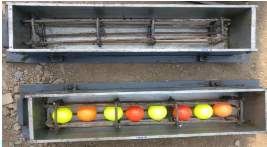
Fig. 2 Form work for Conventional and Bubbled beam
