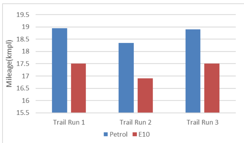
Fig.15 Petrol vs. E10 mileage results on Stock Engine
