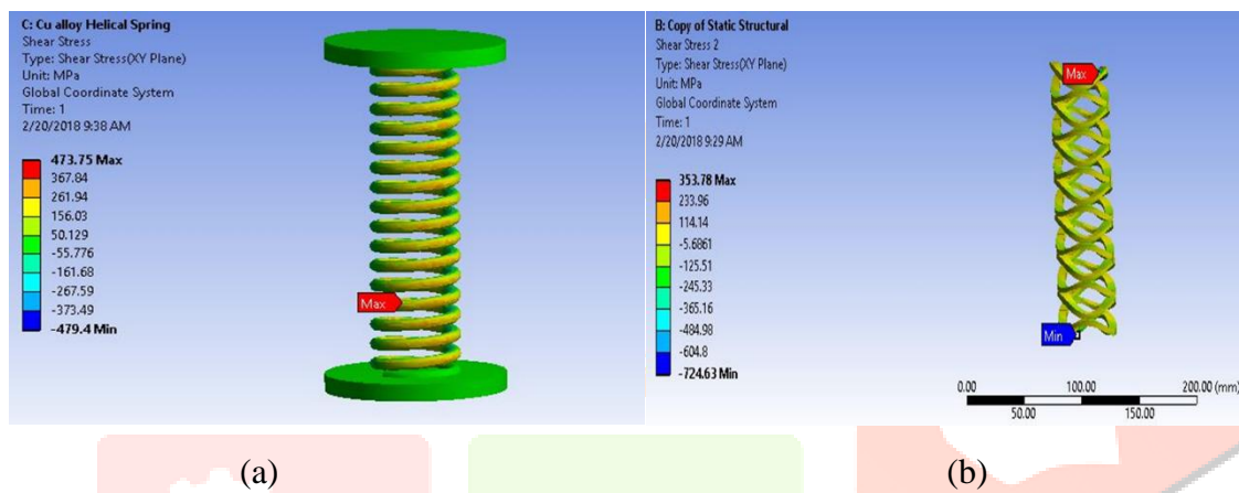
Fig. 5 (a) Shear stress in helical spring (b) Shear stress in wave spring
