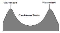
Fig. 5: Watershed segmentation-local minima of gray level yield catchment basins, local maxima define the watershed lines.
