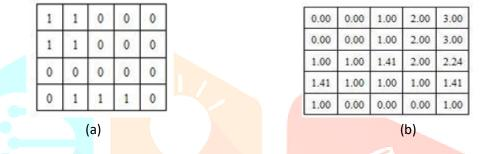
Fig. 6: (a) shows a binary image matrix, and (b) shows the corresponding distance transform G. PRUNING
