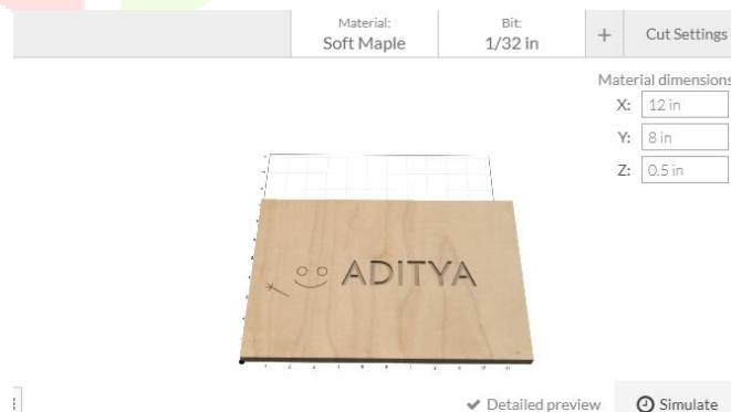
Fig. 4 Milling text by Easel Software
