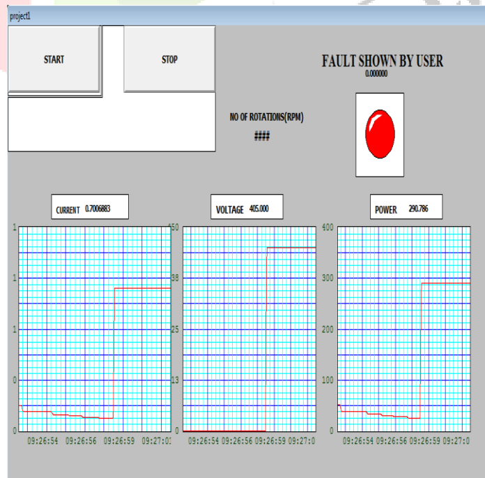
Fig.5: Results obtained from three phase induction motor (1/4 HP) using PLC/SCADA Based Machine Data Enumerator
