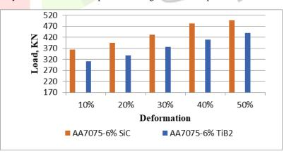
Figure 3.2 Compressive Test
