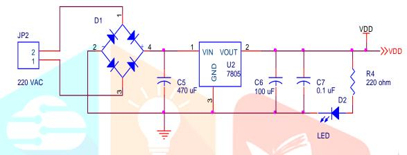
The AC voltage, typically 220V rms, is connected to a transformer, which steps that ac voltage down to the level of the desired DC output. A diode rectifier then provides a full-wave rectified voltage that is initially filtered by a simple capacitor filter to produce a dc voltage. This resulting dc voltage usually has some ripple or ac voltage variation.
