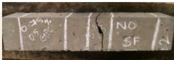
Fig.8 Specimen after testing without steel fibers
