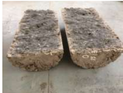
Fig.11. Specimen without steel fibers for split tensile strength test
