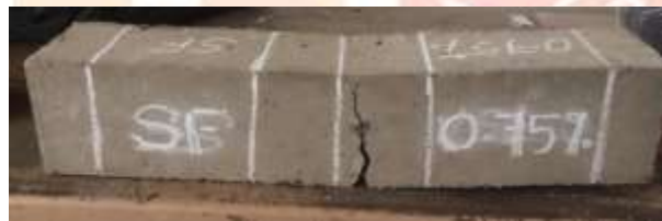
Fig.9 Specimen after testing with steel fibers
