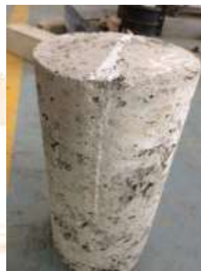
Fig.12 Specimen with steel fibers for Split tensile strength test
