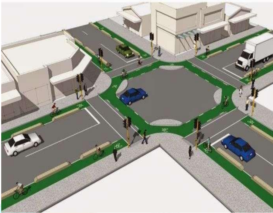
Figure 1 A typical 4 leg Signalized Intersection
