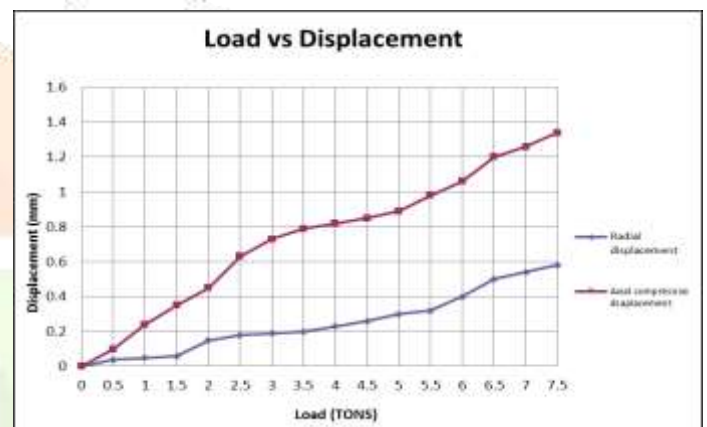
Figure.14: Measure radial & axial displacements
