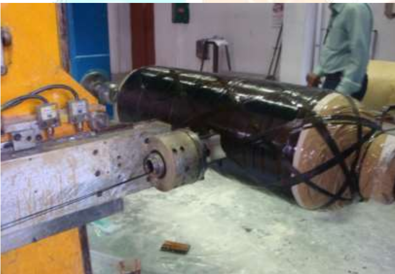
Figure.7: Filament winding of CFRP shell
