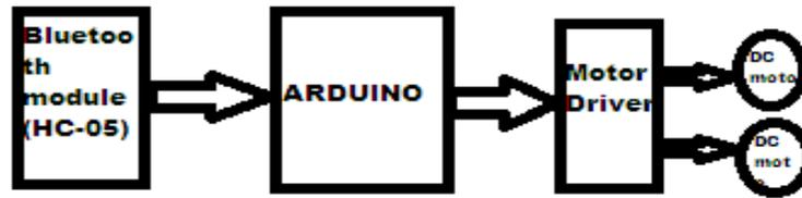
Fig.1 Block Diagram of the Project
