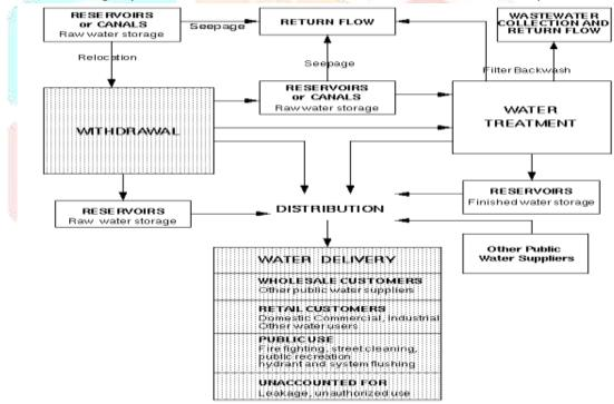
Consumptive use occurs as evaporation from open reservoirs and conveyances. Reservoirs include open and covered reservoirs, tanks and towers.
