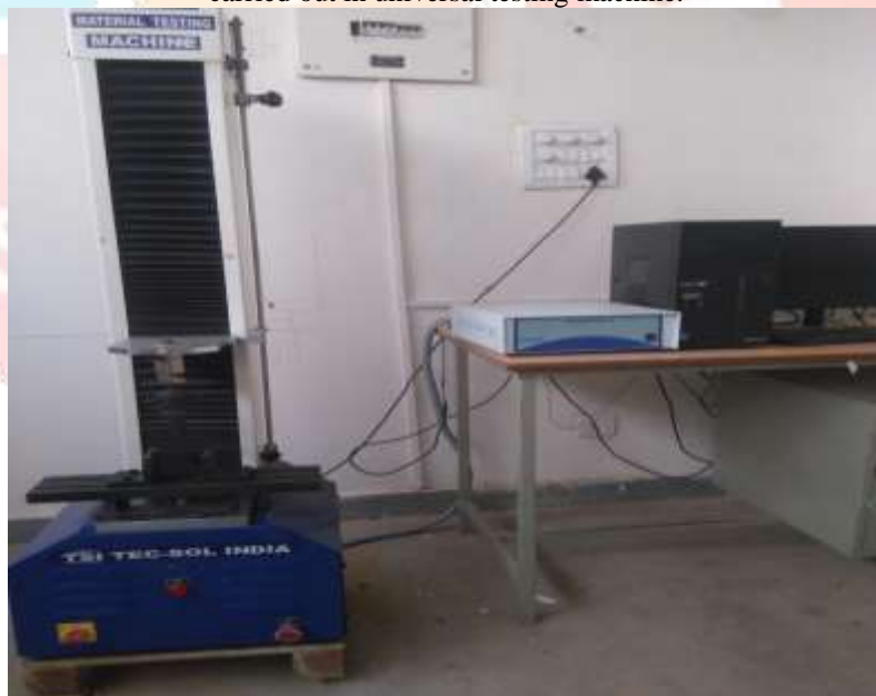
Figure 5.1 Universal Testing Machine used in this project work
