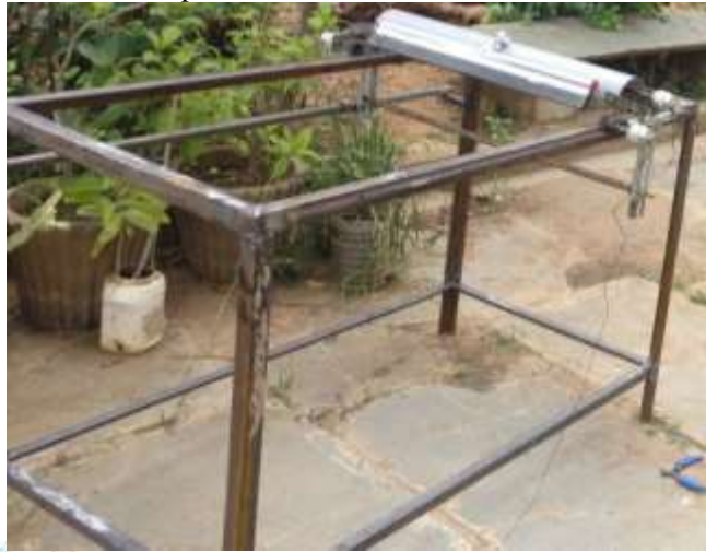
Fig.5. Fabricated electrically operated solar panel cleaner.
