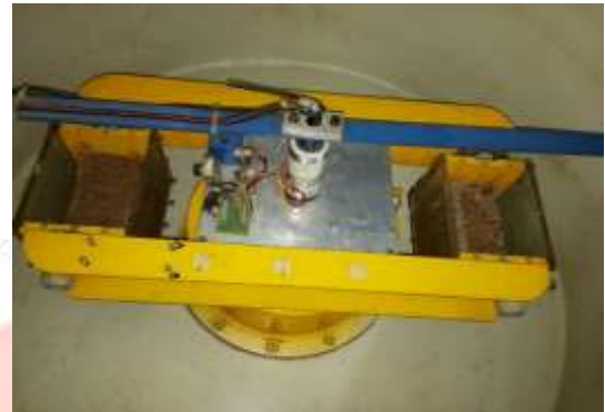
Figure 1.2 (a) GERI Geotech centrifuge machine, (b) Centrifuge as viewed through aperture in chamber roof
