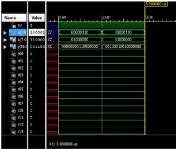
Fig. 6 Output waveform using design 2 in binary format
