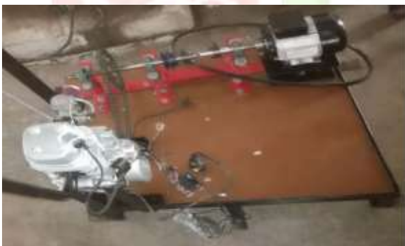
Fig 13- Actual Setup of Engine Operated Power Hacksaw Machine
