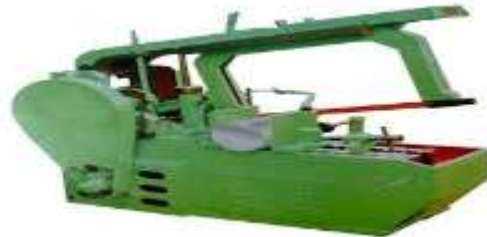
Fig 7- Power Hacksaw Machine
