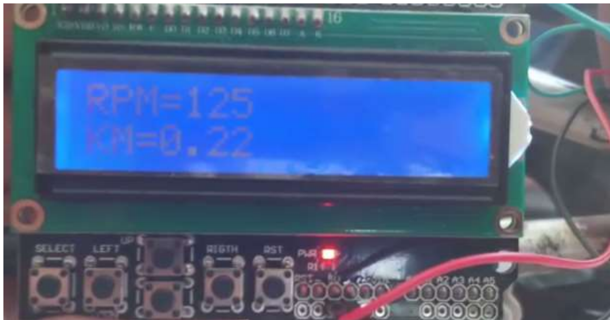
Fig 10: Lcd screen showing rpm and kilometers cycled
