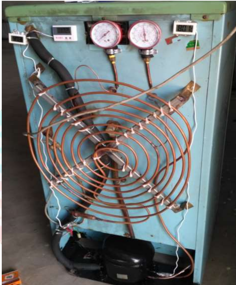
Fig 4: Spiral Condenser VCR Setup
