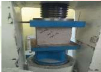
Figure 1. COMPRESSION STRENGTH TESTING
