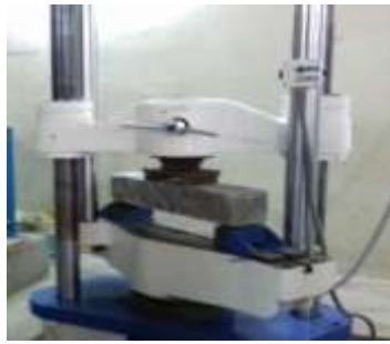
Figure 2. FLEXURAL STRENGTH TESTING
