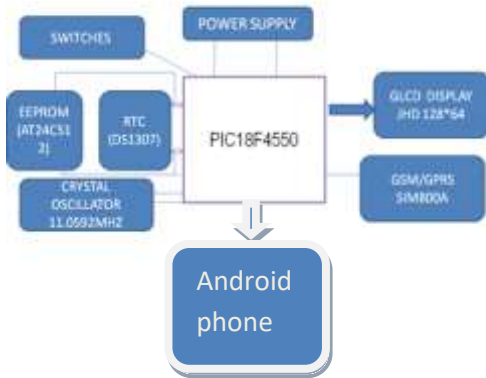
Figure 3. Block diagram of digital notice board
