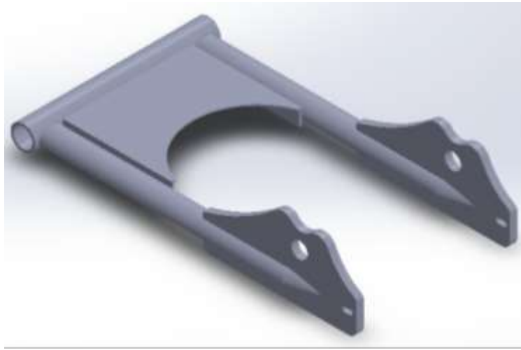
Fig.3. Suspension frame of oval modeled by using solid works
