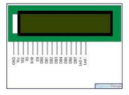
LCD display is Liquid Crystal Display. It is attached along with the arduino board so as to display the readings taken from the crops. The readings may be sensor moisture, humidity or temperature sensor readings for a particular crop.
