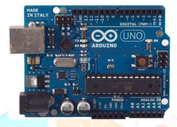
The Arduino microcontroller is an easy to use yet powerful single board computer that has gained considerable traction in the hobby and professional market. The Arduino is open-source, which means hardware is reasonably priced and development software is free. In this project arduino board is used and coding is done in such a way that the robot decides whether the plant needs water or pesticide or both. The inputs for the processing is got from the moisture and DHT sensors
