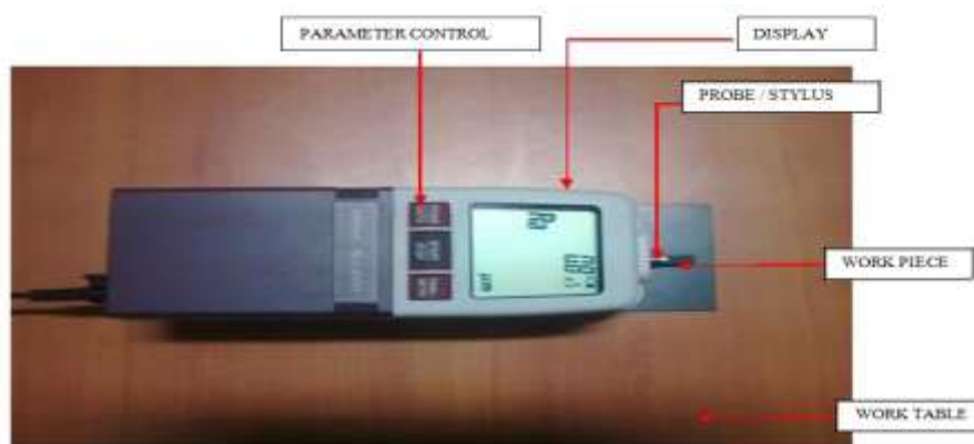
Fig.4 Set Up for Surface Roughness Measurement
