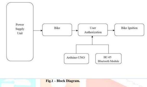
In this block diagram, firstly power supply goes to the bike. After that bike connection check it's authorization through the Arduino-uno, Bluetooth module and RFID for the bike Ignition. Bike has been successfully ignited, when its been successfully.
