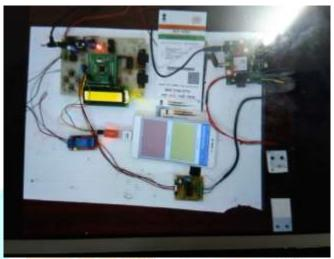
Fig 12. LPC2148 interfaced with peripheral devices along with Application results.
