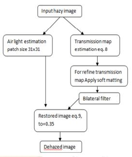
Fig 4: Block diagram for IDCP algorithm
