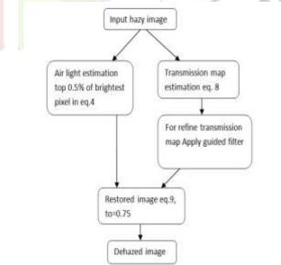
Fig 5: Block diagram for IDCP with guided filter algorithm.
