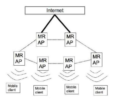
Figure 1: Wireless mesh network
