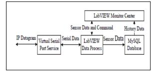
Fig 7. Architecture of Remote Management Platform
