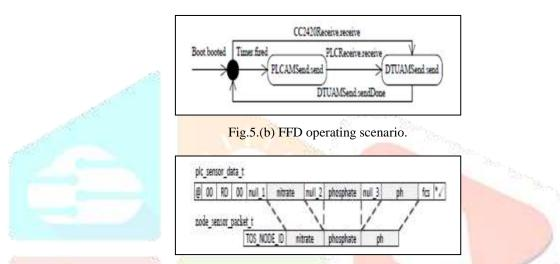
Fig.6. Relationship between plc\_sensor\_data\_t and node\_sensor\_packet\_t.
