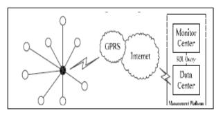
Fig.1. Topology of the network and remote management platform. The disc stands for base station, circle for monitoring nodes.
