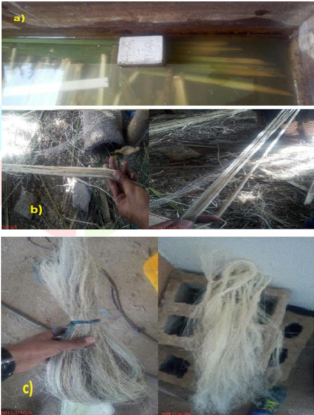
Figure 2. a) Socked papyrus stem b) Manual extraction of fiber c) Extracted papyrus fiber
