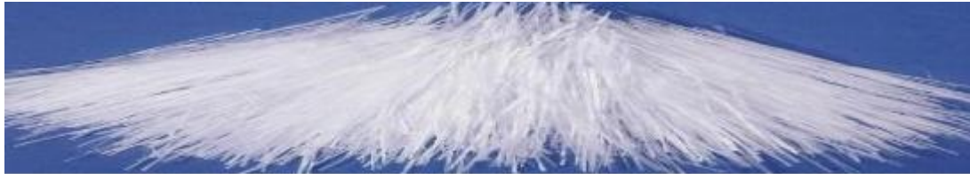
Figure 3. Continuous E-Glass fiber
