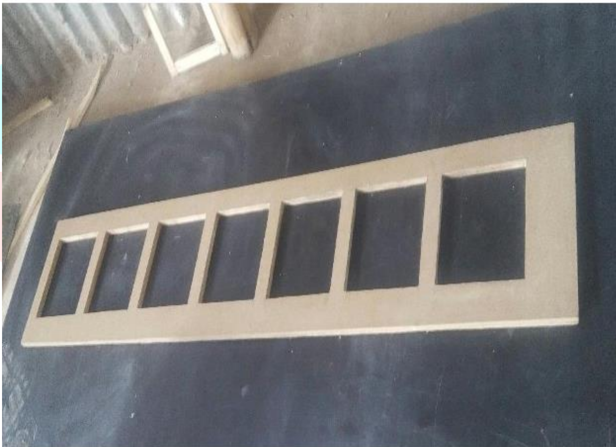
Figure 7. Mould made from rectangular wood
