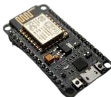
The **NodeMCU ESP8266** module provides wireless communication capabilities to the system. It enables the transmission of real-time energy consumption data from the Arduino Uno to the **Adafruit IO cloud platform** using Wi-Fi connectivity. The ESP8266 acts as an IoT gateway, allowing remote monitoring, data logging, and future integration with smart grid systems. Its low power consumption and integrated TCP/IP stack make it suitable for IoT-based energy applications.
