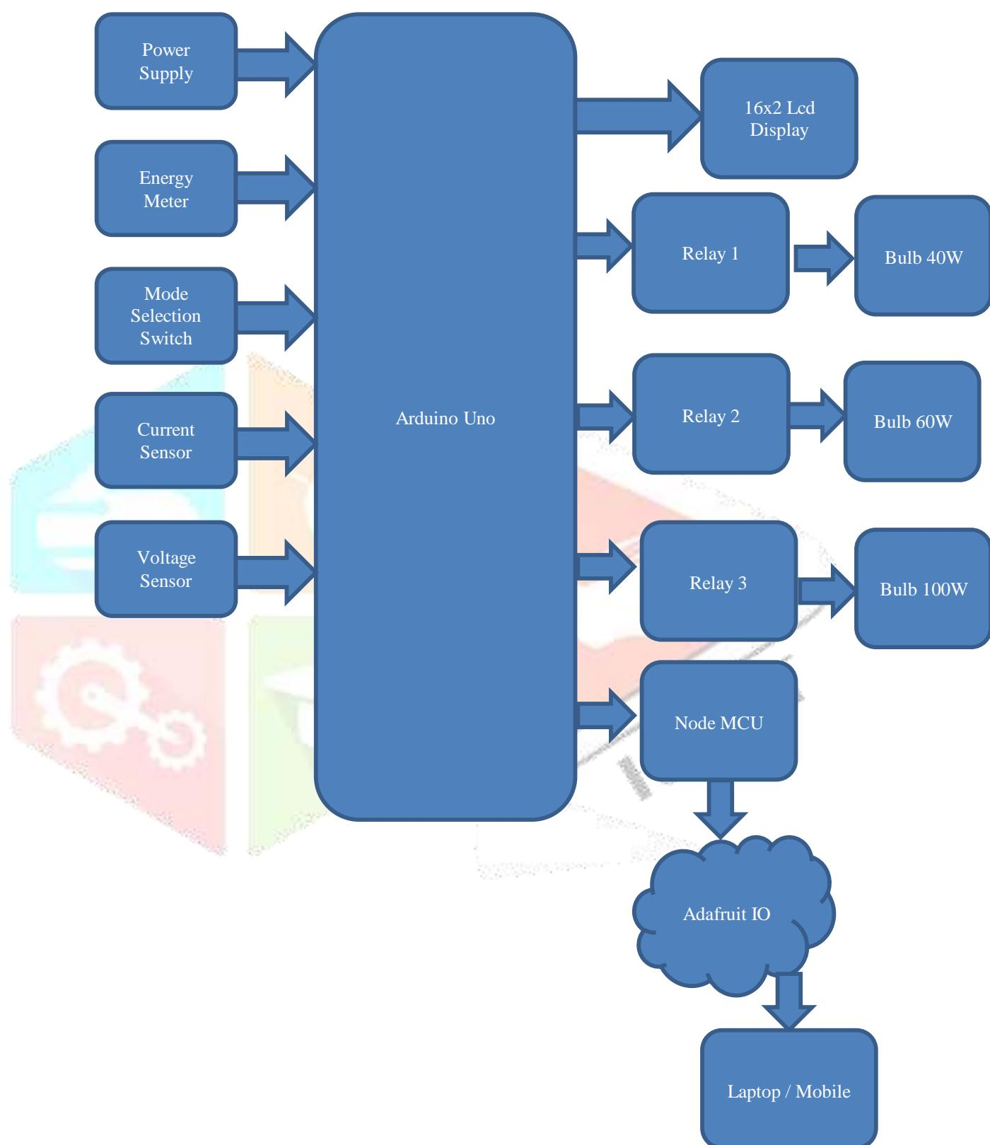
The overall system architecture consists of three major layers: the **sensing and control layer**, the **processing and communication layer**, and the **cloud and user interface layer**.
