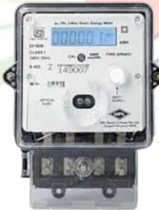
The **energy meter** is used to measure electrical energy consumption accurately. It provides pulses or digital outputs proportional to the consumed energy units. These signals are interfaced with the Arduino Uno, which converts them into energy units (kWh) through software calculations. The energy meter ensures reliable long-term measurement and acts as the primary reference for billing in both prepaid and postpaid modes.
