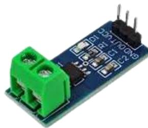
The **current sensor** continuously measures the load current drawn by connected electrical appliances. It provides an analog output proportional to the current flowing through the circuit, which is read by the Arduino's analog input pins. Accurate current measurement is essential for real-time power calculation, load monitoring, and detection of abnormal consumption patterns. The sensor enhances system safety and measurement precision.
