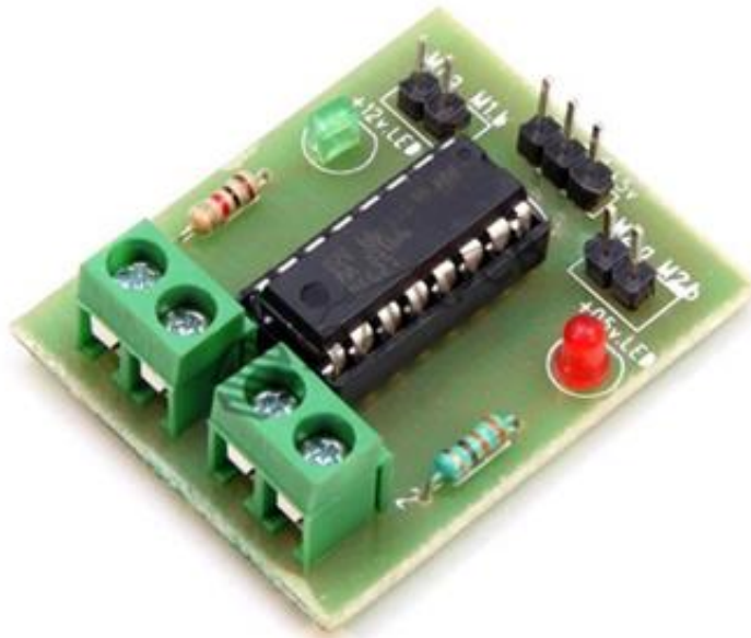
Fig4.2.7. L293D motor controller
