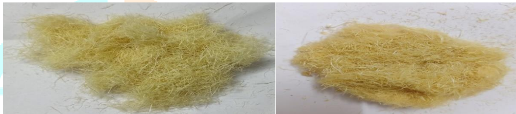
Fig.1 (a) untreated PJ fibers Fig.1 (b) PJ fibers after alkali treatment
