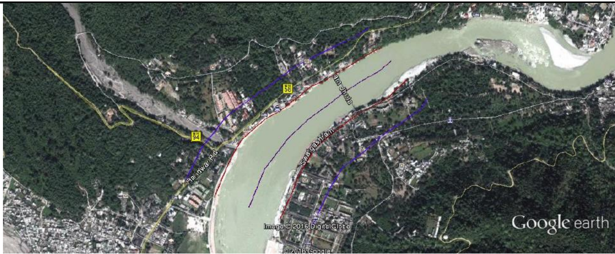
Fig. (3): River Center Line, Bank Line and Flow Path in Google Earth Pro at Ramjhula for Ganga River
