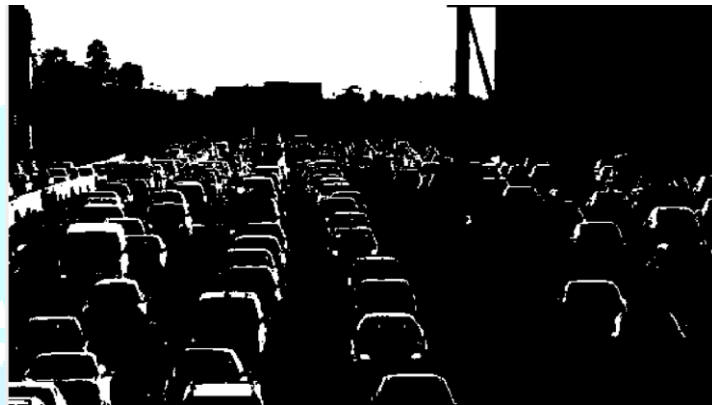
Figure 10 Segmented frame of Downloaded video by the method of Thresholding
