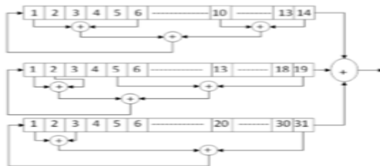
Fig 4: PN Sequence generator
