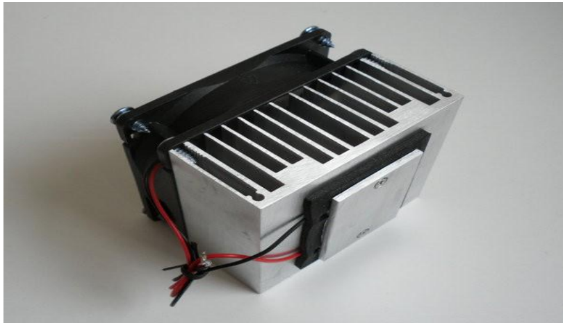
fig 5 heat sink with cooling fan
