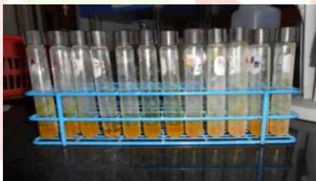
Plate:3 Reducing sugar analysis by DNS method
