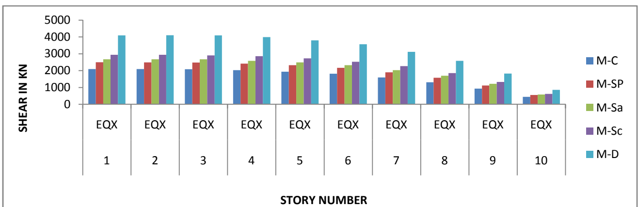
Fig-9 Max story shear of 10 story conventional, shear walls and diagrid arrangements
