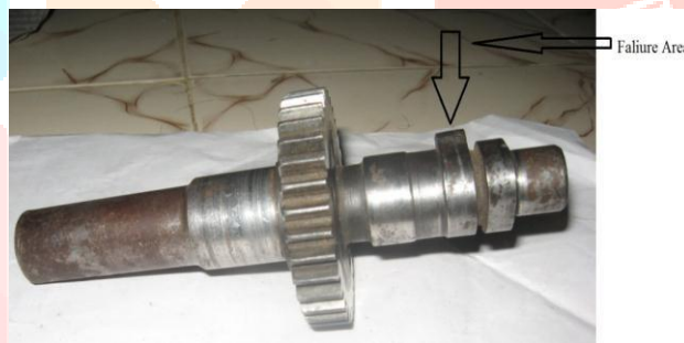
Figure 1 Failure of the Camshaft
