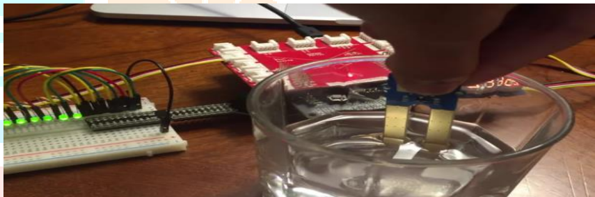
Fig 3.3 Moisture Sensing LED Gauge
