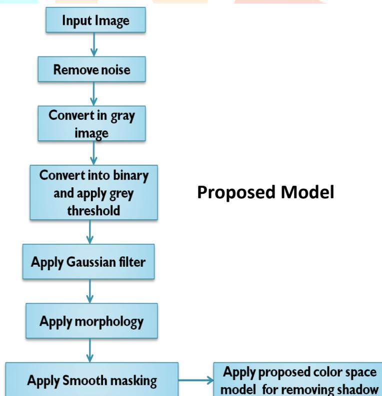
Fig-3 Proposed Algorithm flowchart
